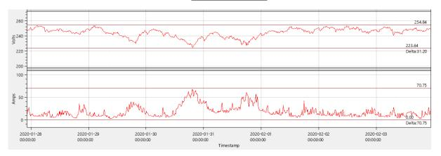
VRDT Installed: V = 236-246 V<sub>rms</sub> - COMPLIANT
