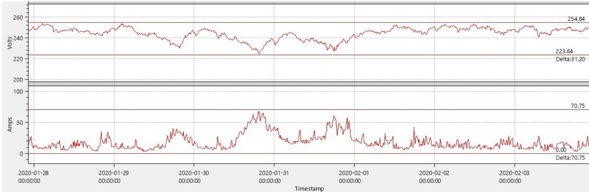
VRDT Installed:  $V = 236\text{-}246\text{ V}_{\text{rms}}$  **COMPLIANT**
