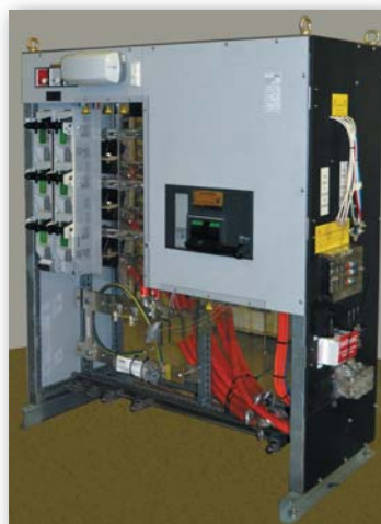
1000kVA 11kV substation to electrical utility specification. Elongated style in Stainless Steel enclosure with 4-way RMU and LV board with C/B. Designed and produced in Mittagong, NSW.
