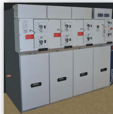
EFACEC 12/24kV 4 way unit with 3 switch functions and 1 fused transformer function. Test bushings accessible under covers on front at top
