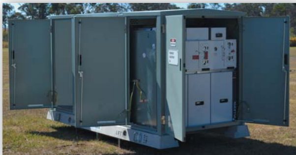
1000kVA 11kV substation to electrical utility specification. Elongated style in Stainless Steel enclosure with 4-way RMU and LV board with C/B. Designed and produced in Mittagong, NSW.
