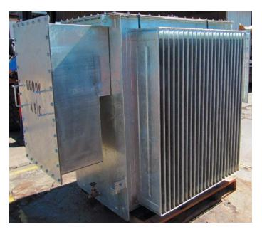
Typical applications will have LV and HV cable boxes with removable gland plates. Bolt on or fixed radiators in galvanized or painted finish can be supplied to meet the cooling requirement of the site. OTI, PRV's, WTI, OLI are all common fitment, prewired to a convenient marshaling box for the customers connection.
