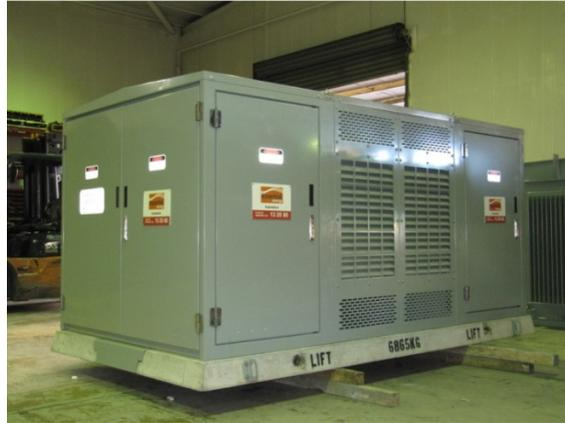
Complete 1000kVA 11kV substation to Essential Energy specification. Elongated style in Stainless Steel enclosure with 4-way RMU and LV board with C/B. Designed and manufactured by Tyree in Mittagong, NSW.
